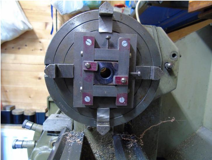
The 4-jaw chuck was carefully adjusted to ensure that the pop mark was running true. The axlebox hole was drilled, bored and reamed to size. I always use a small boring tool before reaming to ensure that the finished hole is correctly positioned.
