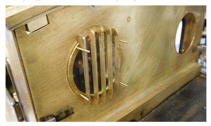
Don Young says to "press fit" the spectacles in the holes, but the real ones actually hinge at the top; there's a catch in the cab roof so that they can be swung up inside and latched in the open position – see below. And no, I'm not doing that. I will solder some little pieces of brass sheet (fixed dummy hinges) on to the inner rings as per the real one and just screw them on to the cab, front and back.
