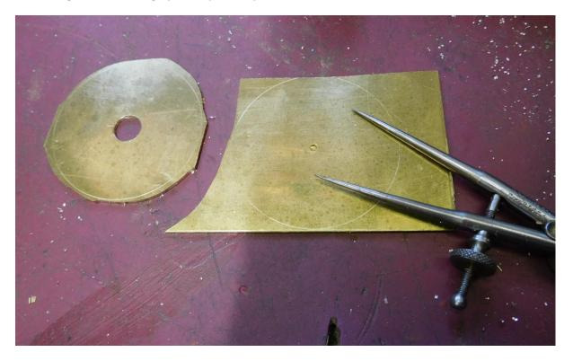
I used a step drill to form an 8mm hole in the middle of each one...
