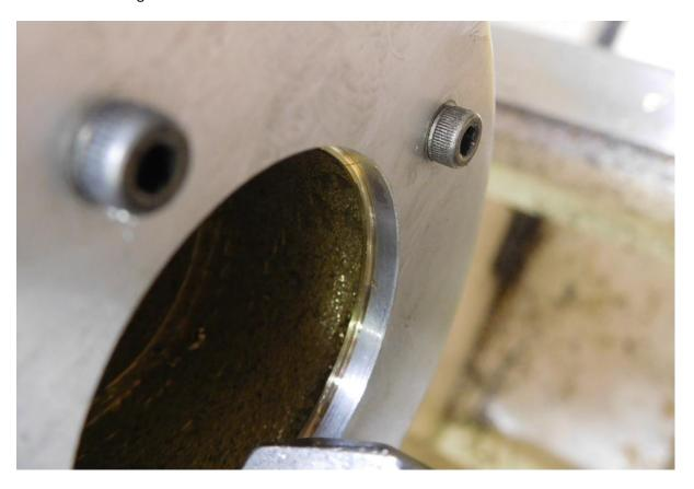
Then I needed to hold it by the *inside*, so I made another fixture from aluminium, slotted as shown with a hacksaw; tightening the countersunk M8 screw expands the fixture to grip the inner diameter securely – hence why I made them as near to size as possible. I had to machine a substantial groove behind the locating diameter down to about 12mm in order for the fixture to expand without having to put a six-foot pipe on the Allen key to secure it.
