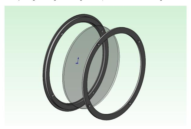
So do I make them out of a piece of brass bar, or cut them from sheet? Sheet won as it was much less wasteful of brass. Beside, Hoapit Works was a bit short of 1¾" dia brass bar... I marked out a circle on some 1,2mm brass sheet and cut eight of them roughly to shape on my bandsaw...
