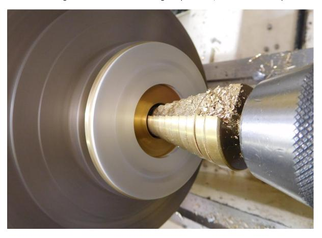
One step-drilled out, and the next one waiting. At the same setting I bored out the middle to 34mm as accurately as I could with a boring tool. (Yawn...)
