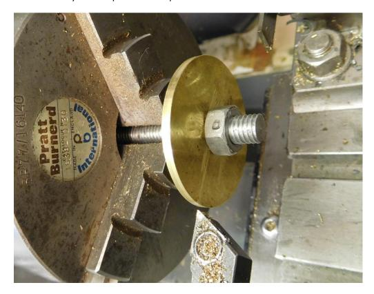
Next step was to make a turning fixture. You haven't a hope in hell of holding 1,2mm thick brass sheet of these dimensions in a chuck because if you tighten the chuck sufficiently to stop the job flying off somewhere when the tool hits it, you distort the job and it ends up looking like an Austin Allegro steering wheel rim... Remember those?
