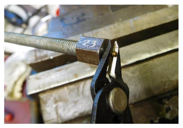
Then the thing was popped in the lathe and the screw faced to length. A needle file would take care of any rough threads if necessary – if there's enough thread peeping out! Give your screw the maximum support you can; you should be working as close to the end face of the "nut" as possible.
