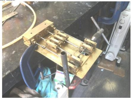
More of what the micro welder can do arose while trouble shooting the connecting rods because they had to have split big ends and, having made and fitted them to the crankshaft, I realised that the eccentric straps were large in relation to the con rod big ends, so I will have to make daintier ones. (There is nothing like experience).
