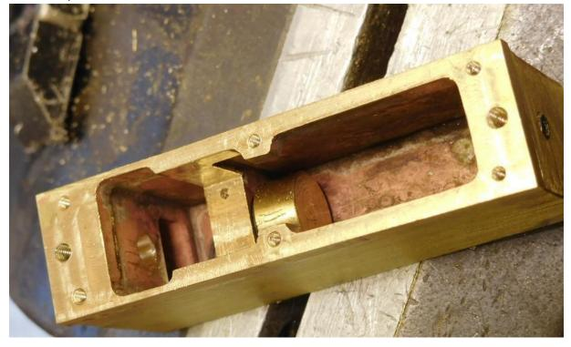
Here's the plug after use; you can see how awkward the M2 holes would have been to drill and tap, without supporting it with the plug:
