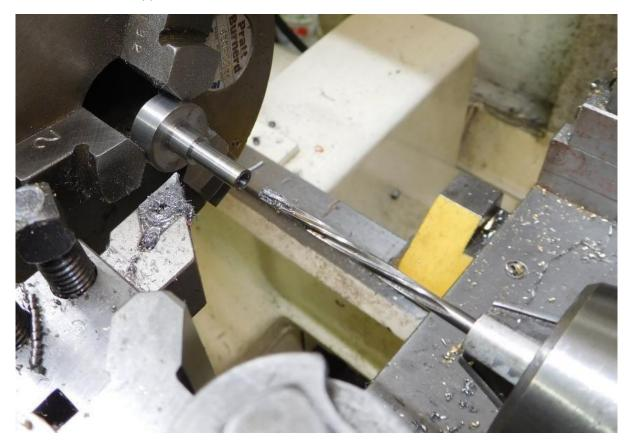
I fitted the drill jig to the lubricator and drilled the new insert 3,1mm:
