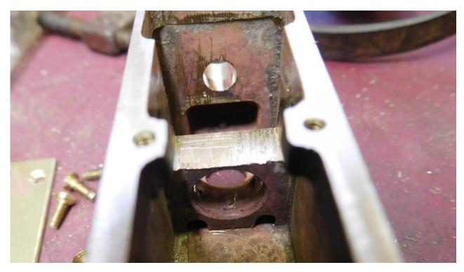
Having finished the cutout, I made the new insert piece and I now needed to secure it to the remains of the old outrigger with two M2 cap-head screws. Now there was an existing hole in the outrigger (Green on the CAD illustration above, and fairly obvious in the photo above). This is to allow oil to flow from the filler into the pump area, and those two M2 tapped holes I needed were just going to collide with it at a nasty angle. Cue broken drills and/or M2 taps and more "Grrrr!" noises.
