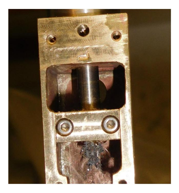
The insert was stamped to ensure it subsequently gets refitted the right way round; I was pleased I'd made the insert accurately enough so that it fits either way, but once the 1/8" hole was in place, there's probably only one right way now!
