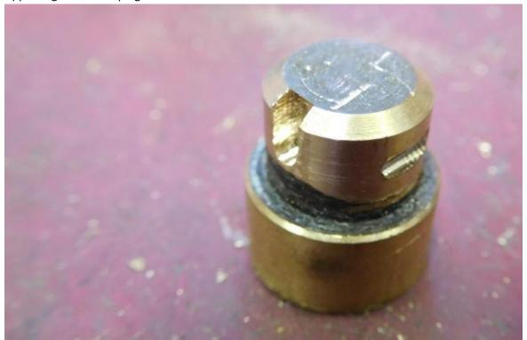
Next, I needed to produce the 1/8" bore in the new insert for the crank bearing. It needed to line up very accurately with the existing 9/32" outer hole.
