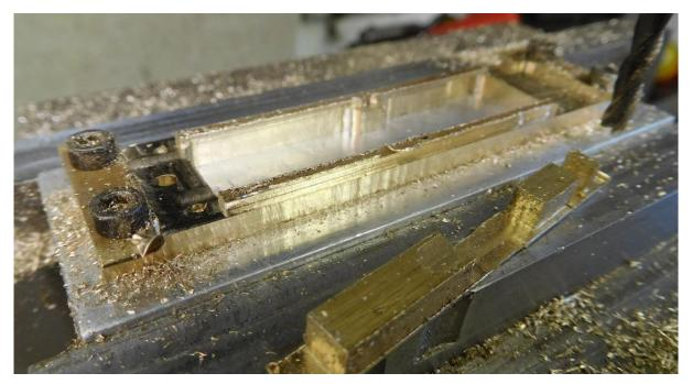
The over-long bits at each end (with the holes for the cap-head screws securing it to the fixture) were cut off slightly oversize for machining back to match the rest of the lubricator after final brazing. Besides, having the ends stick out a bit helped with feeding in the solder during brazing.
