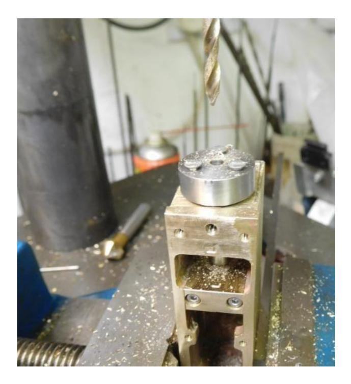
...then following up with an 1/8" reamer. The steel swarf on the end of the reamer is from the drill jig, which was sacrificial in that you don't normally machine the jig!!
