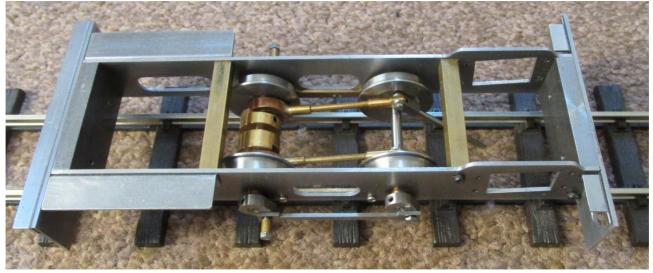
Those of you familiar with this design will spot that I have changed the eccentric straps from the spit type to solid circular ones. This was for simplicity of machining but needs the compensating move of a bolted pivot in the valve rod to permit the easy dropping of the wheels, the original two parts of the valve rod being assembled by rivetting.
