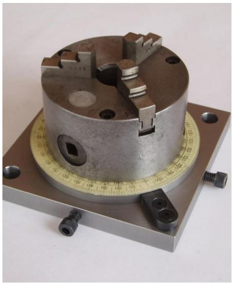
would use a beefier rotary table so there would be no danger of the milling cutter snatching and trying to lift the whole thing off its base.
