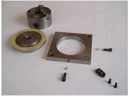
The graduations are provided by a modified plastic 360 degree protractor, stuck in place with epoxy and also clamped by the chuck as it bolts down. Note the brass pads under the clamping screws; these are to prevent bruising of the chuck spigot which may make it stiff to turn. The chuck itself is 3 ¼ inches diameter, to give you an idea of scale.
