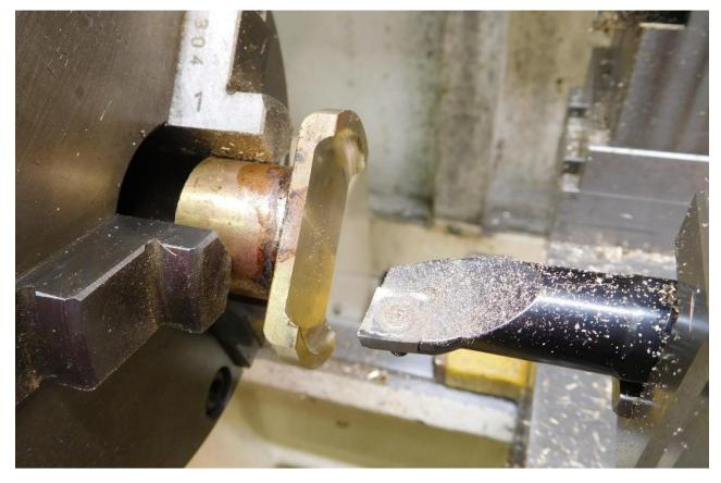
Same process was used for the external radius, but using a parting tool, which could get into the gap between the chuck jaws and job. You can just make out the steps here – they're 0,25mm increments. (About ten thou...)
