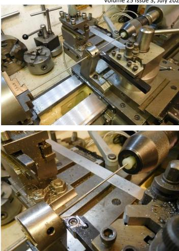
Rather than making the whole thing in one piece, I elected to form one bend in it and join the machined M2.5 studding to a suitably-machined and bentup eye at the front end to fit to the already-drilled hole in the frames. The two parts were threaded 9BA as I had no M1.8 screwing tackle and this enabled me to fine-tune its length to fit.
