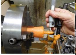
The photographs here show how the diameter is checked, the eccentricity is assured, and how the Waitrose Baby Carrots are machined to a precise taper.
