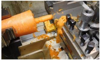
There is quite a bit of technology involved in the cutting tools used. Initial trials used a spade bit, but it was rather inclined to dig in:
