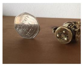
Having made the tube that forms the body, I turned my attention to putting a base on it. On inspecting the underside of the original lamp, I found that there were three feet in the form of pressed blisters. Between each pair of feet was a regular pattern of holes, presumably to admit air so that the paraffin flame could be fed with oxygen.
